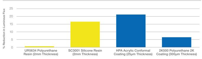
Protection Media Applied at Typical Application Thickness
